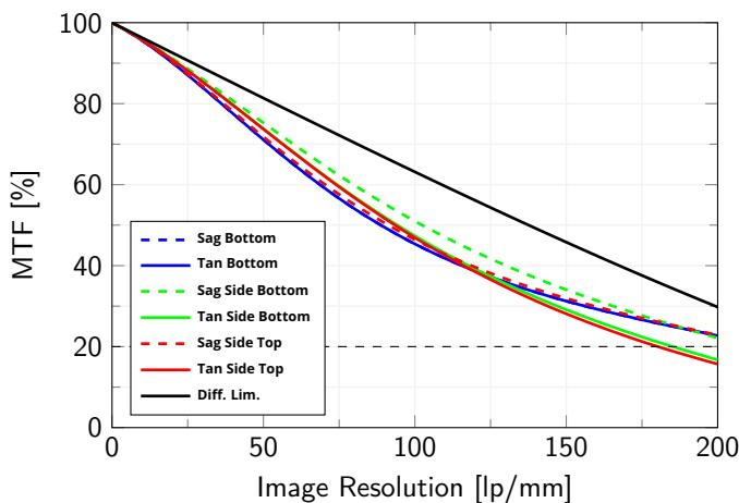
Modulation Transfer Function (MTF) vs. Image Resolution (wavelength range 486 nm - 656 nm),  $wf/N = 5$ , of cylindrical object of diameter 30 mm and height of 20 mm
